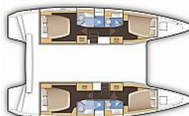
Deck on Deck-Plan: Lagoon 42 catamaran / 4 water tanks
