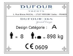
The Builder's identification plate is located in the cockpit. It carries important information, which is explained below.
