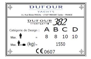
Some of this information is provided on the builder's plate attached to the boat. A full explanation of this information is given below.
