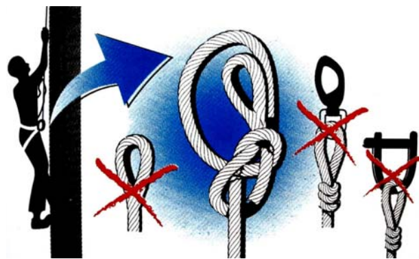
Advice for hoisting a person up the mast
