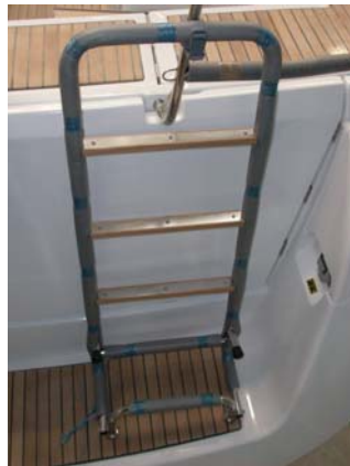
Swimming ladder (means of coming back onboard)
