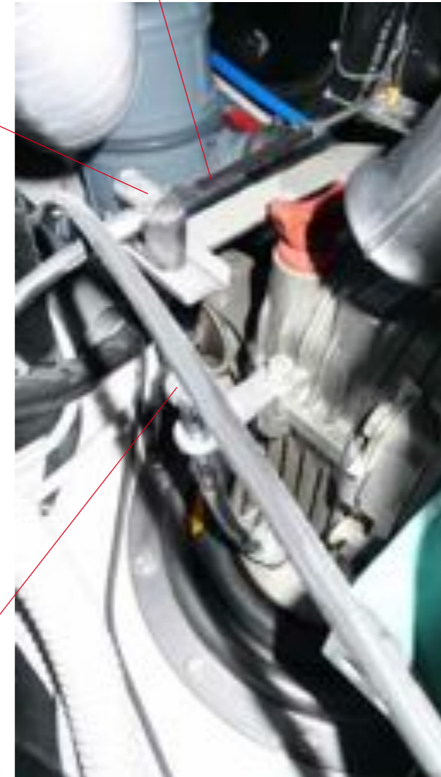
THROTTLE CABLE SHEATH BLOCKING DEVICE
