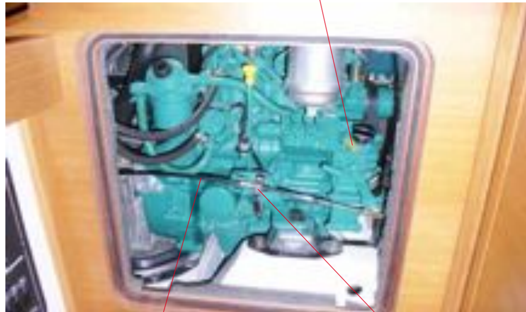
THROTTLE CABLE SHEATH BLOCKING DEVICE
