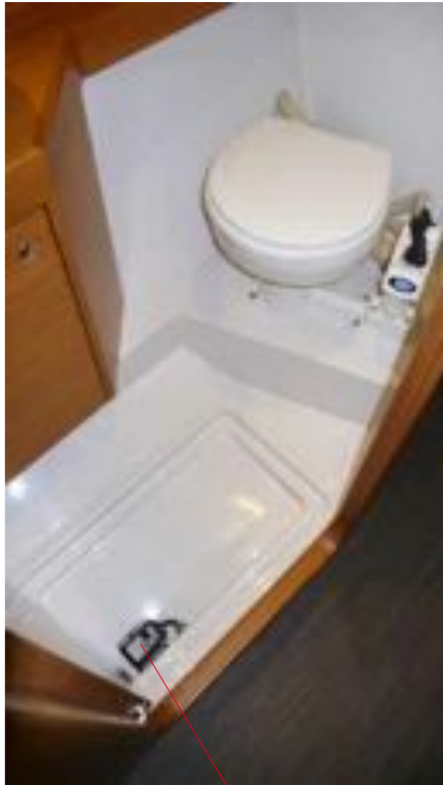
SHOWER SUMP LEVEL SENSOR FOR PUMP OPERATION
