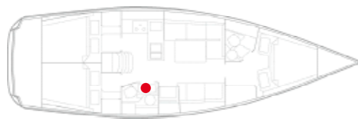
SHOWER SUMP LEVEL SENSOR FOR PUMP OPERATION
