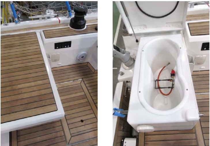
Gas cylinder locker
