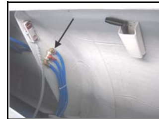
Selection valve - Fresh water / Sea water (Reference 4)
