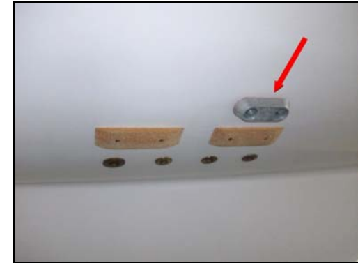
ANODE (On hull, under water line)
