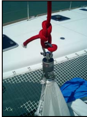
FIXING OF THE GENNAKER HALYARD ONTO THE HEAD
