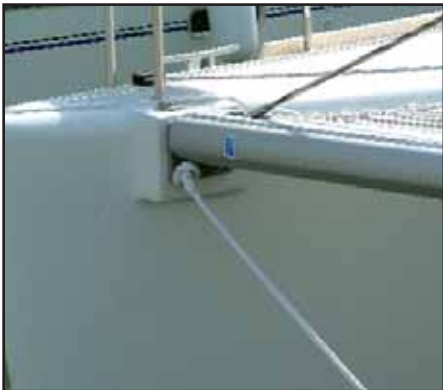
ATTACH THE BRIDLE TO THE FORWARD BEAM
