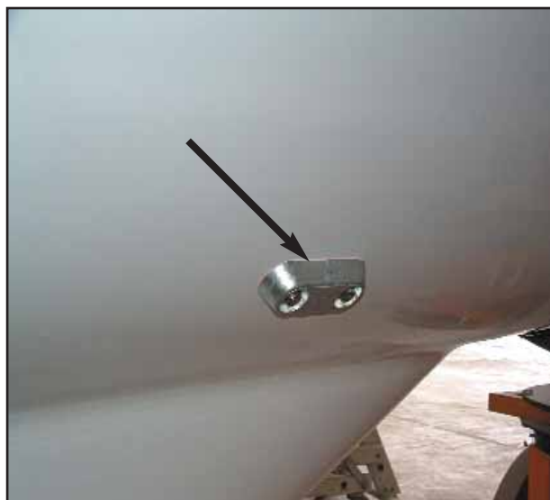
ANODE (On hull, under water line)
