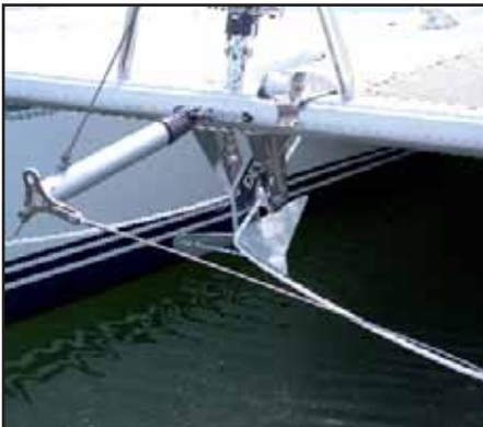
RUN THE BRIDLE THROUGH THE BOW ROLLER
