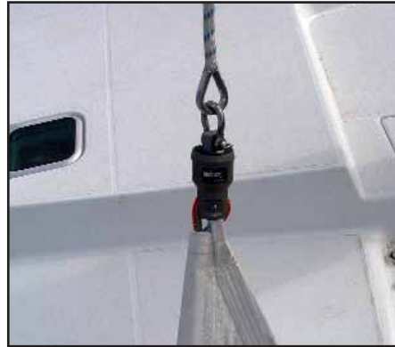
FIXING OF THE GENNAKER HALYARD ONTO THE HEAD
