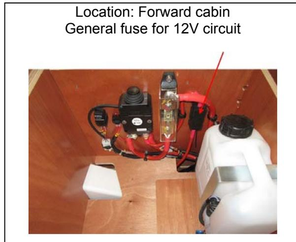
When replacing fuses/circuit-breakers, always ensure replacements are of the correct capacity (see the colour-codes)
