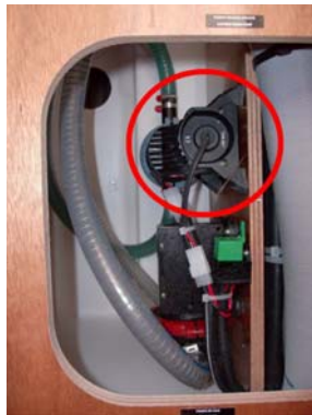
Draining pump for shower - Under the companionway
