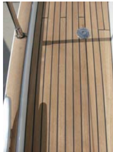
WC evacuation Deck Location Filler cap Passageway Port side
