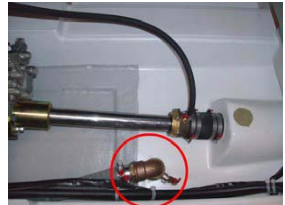
Sea water inlet valve for engine (Reference 3)
