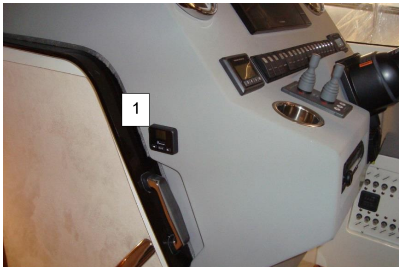
Picture 54: The heater switch (1)
