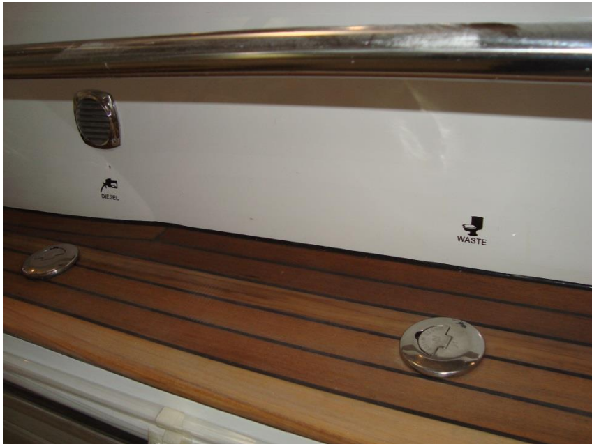
Picture 50: Location of deck discharge
