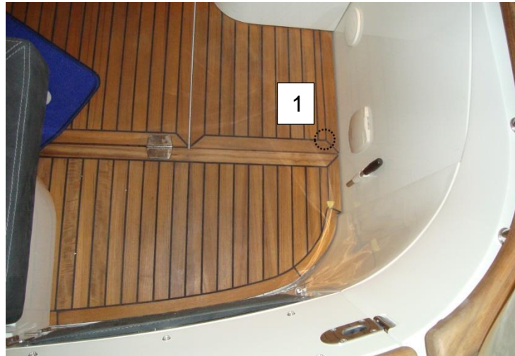
Picture 15: Aft deck drain on the starboard side (1)
