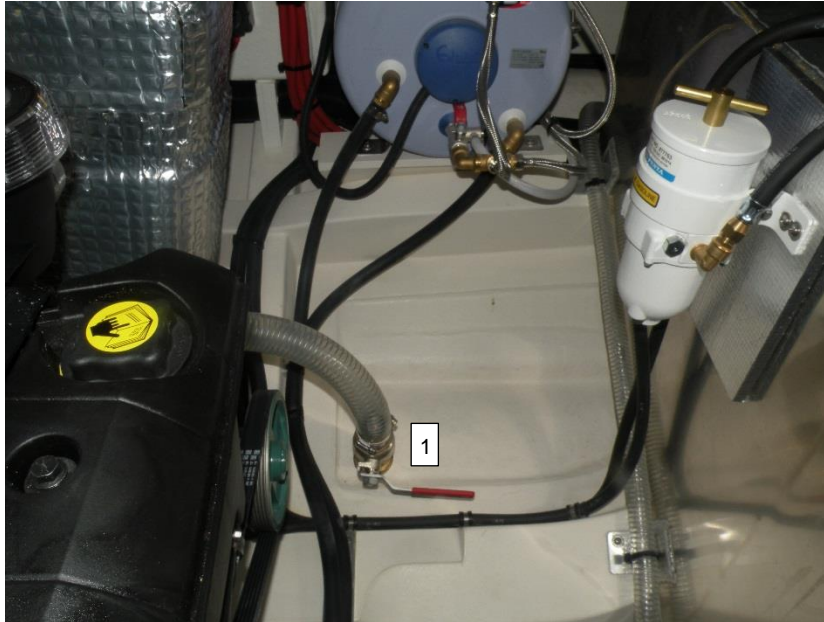
Picture 12: Location of seawater inlet for engine cooling and Closing valve (1) (optional)
