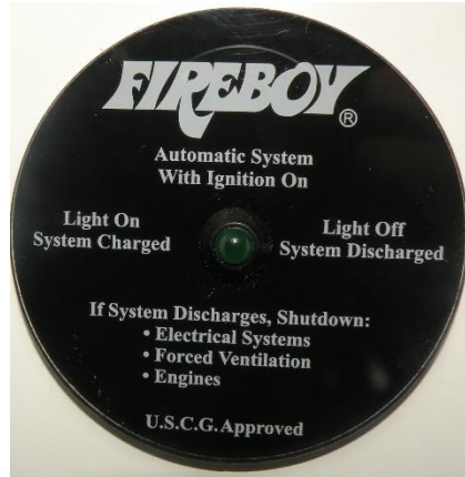
Picture 5: Fire extinguisher indicator
