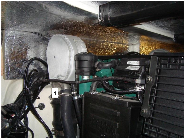
Picture 31: The exhaust hose (1)
