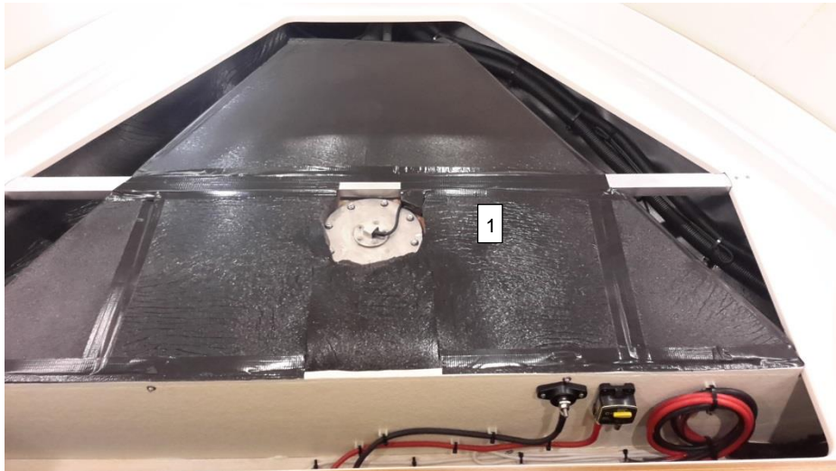
Picture 22: Fresh water tank in the front cabin – under the front bed (1)
