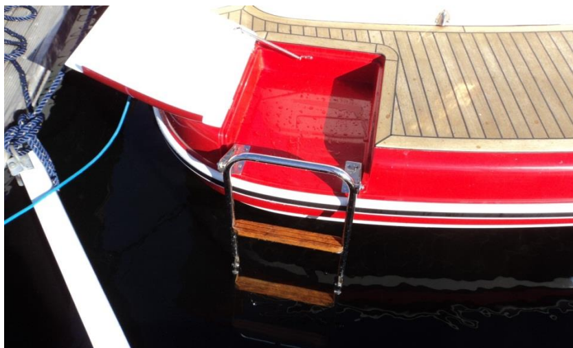
Picture 13: Bathing platform with open ladder cover
